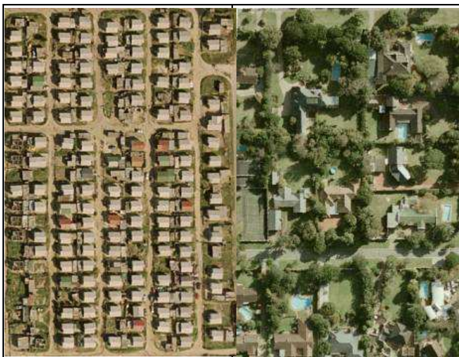
Figure 6. Comparison of dwelling density between the low-cost settlement at Motherwell NU 31 (left) and affluent Walmer (right). The left image contains 168 dwellings on 3.66 ha while the right image contains 15 houses on the same area of land. Note how trees and bushes in Walmer provide microhabitat for fauna and that there are no trees present in the township.
